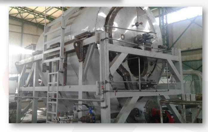
New technology as our equipment has been installed and tested to ensures high quality at the same time there are no emissions into the atmosphere Thermal conversion of biomass (rice straw) to Biochar through pyrolysis process in the absence of oxygen Environmental Friendly equipment
